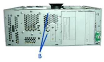
Figure 4 - 17 : HDD Bracket Screws
